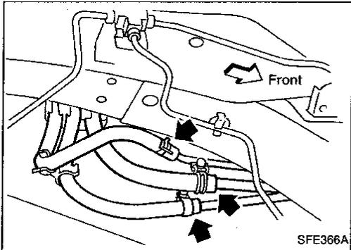
4. Disconnect fuel tubes located on the lower right-hand side of fuel tank.
