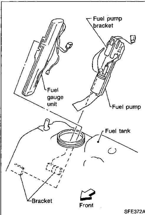
6. Remove fuel pump pulling the top end of the fuel pump bracket upward.
