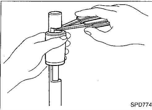
10. Set aside the selected correct pinion bearing preload adjusting washer. Use it when assembling the pinion gear and bearings into the final drive.
