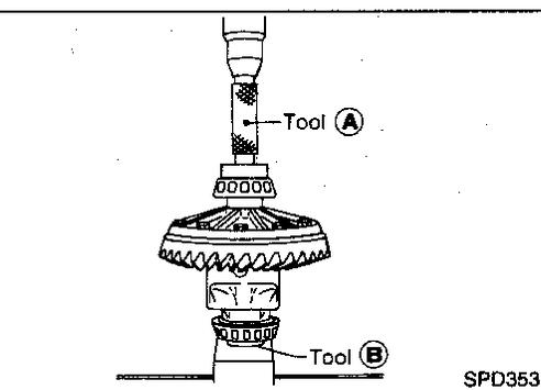
4. Press-fit side bearing inner cones on differential case with Tool.
