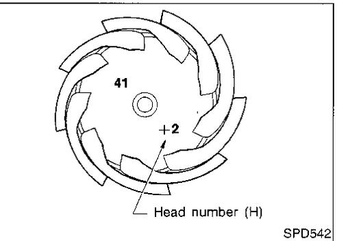
14. Correct the pinion height washer size by referring to the "pinion head number".
