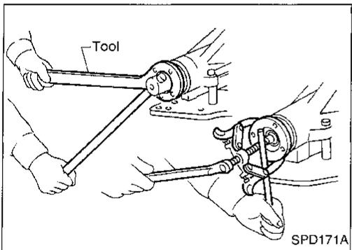
6. Take out drive pinion (together with rear bearing inner race, bearing spacer and adjusting washer).
