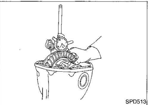
14. Measure ring gear to drive pinion backlash with a dial indicator.
