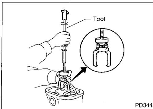
**Keep the side bearing outer races together with inner cone — do not mix them up.**
