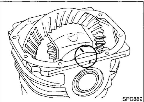
2. For proper reinstallation, paint or punch matchmarks on one side of the side bearing cap.
