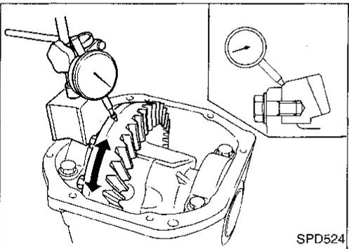
13. Check runout of ring gear with a dial indicator.
