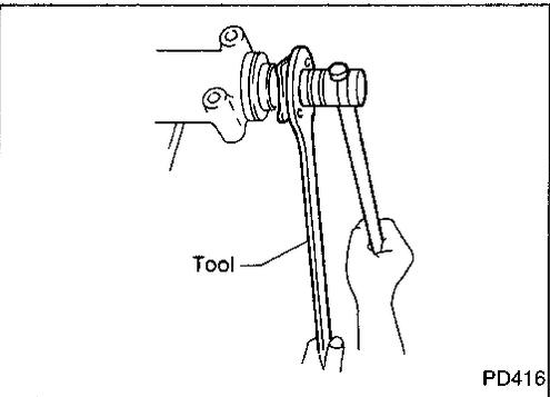
7. Install companion flange, and tighten pinion nut to specified torque with suitable tool.
