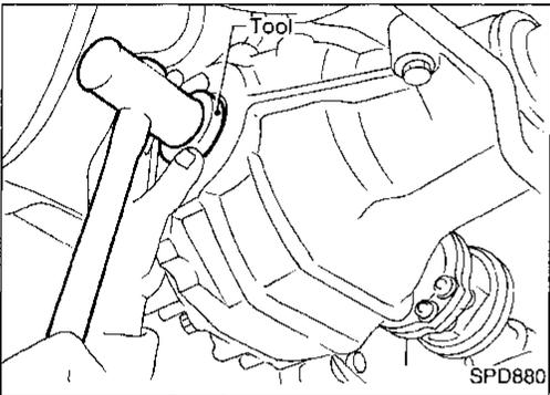
4. Apply multi-purpose grease to sealing lips of oil seal. Press-fit oil seal into carrier with Tool.
