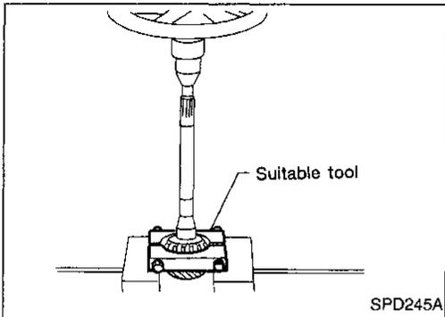
11. Remove pinion rear bearing inner race and drive pinion height adjusting washer with suitable tool.
