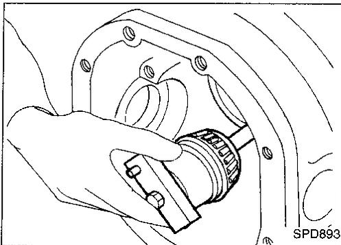
3. Install the pinion rear bearing inner cone into the final drive housing. Then place the pinion preload shim selector Tool, J34309-1, gauge screw assembly.
