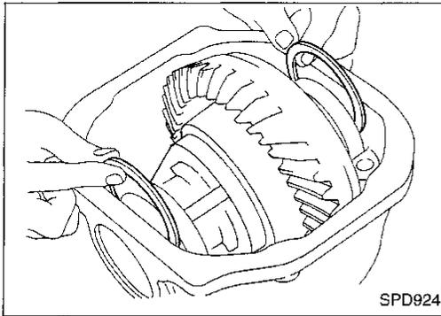
10. Insert left and right side bearing adjusting washers in place between side bearings and carrier.
