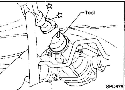
5. Apply multi-purpose grease to sealing lips of oil seal. Press front oil seal into carrier.
