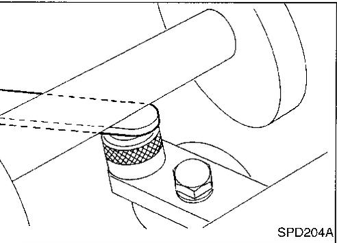
12. Select the correct standard pinion height adjusting washer thickness. Select by using a standard gauge of 3 mm (0.12 in) and your J34309-101 feeler gauge. Measure the distance between the J34309-11 pinion height adapter including the standard gauge and the arbor.
