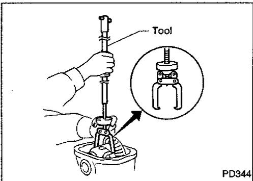
10. Remove the carrier from the final drive housing. Save the selected preload washers for later use during the assembly of the final drive unit.
