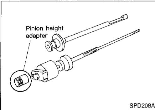
7. Place the J34309-11 "R200A" pinion height adapter onto the gauge plate and tighten it by hand.
