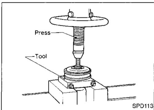
5. Remove center bearing with Tool and press.
