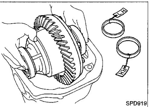
9. Install differential case assembly with side bearing outer races into gear carrier.
