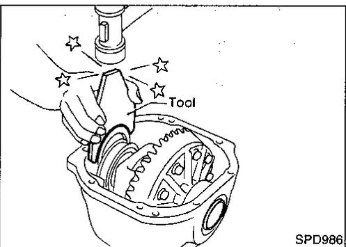
4. Use the J25267 side bearing spacer drift. Place original carrier side bearing preload shims on the carrier end, opposite the ring gear.
