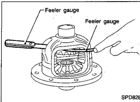
3. Adjust clearance between rear face of side gear and thrust washer by selecting side gear thrust washer. Refer to SDS (PD-33).
