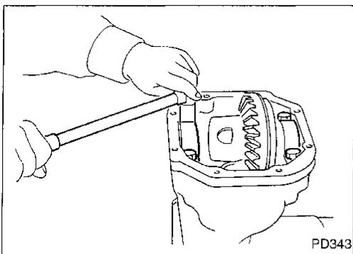
4. Lift differential case assembly out with Tool.
