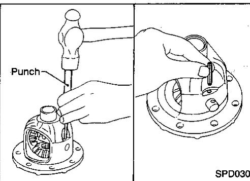
1. Install pinion mate shaft lock pin with a punch. —R200 ONLY—
