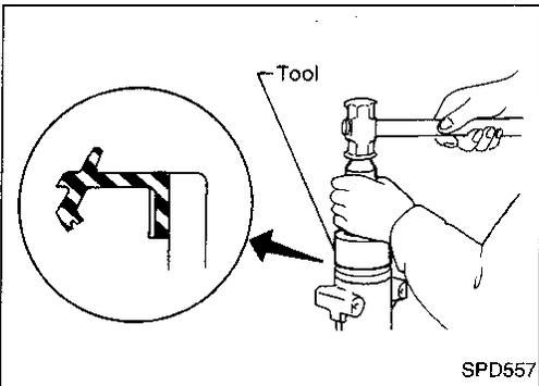
6. Apply multi-purpose grease to cavity at sealing lips of oil seal. Install front oil seal with Tool.
