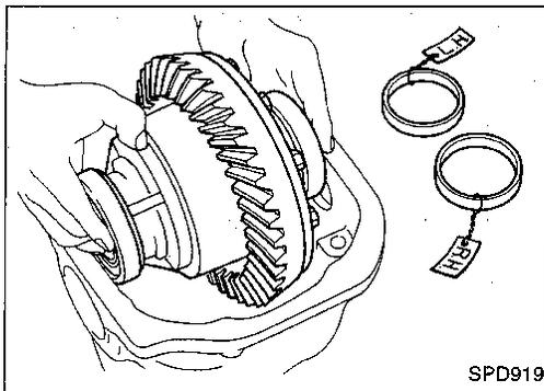
1. Make sure all parts are clean. Make sure, also, the bearings are well lubricated with light oil or DEXRON™II type automatic transmission fluid.
