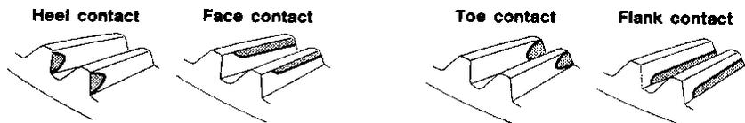
To correct, increase thickness of pinion height adjusting washer in order to bring drive pinion close to ring gear.
