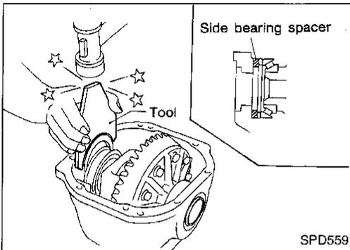
11. Drive in side bearing spacer with Tool.
