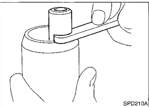
9. Select the correct thickness of pinion bearing preload adjusting washer. Select by using a standard gauge of 3.5 mm (0.138 in) and your J34309-101 feeler gauge. The exact measure you get with your gauges is the thickness of the adjusting washer required. Select the correct washer from the following chart.
