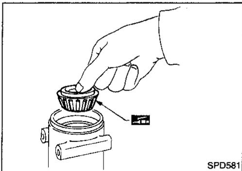
5. Set drive pinion assembly (as shown in figure at left) in differential carrier and install drive pinion, with press and suitable tool.
