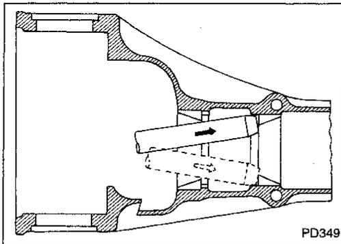
10. Remove pinion bearing outer races with a brass drift.
