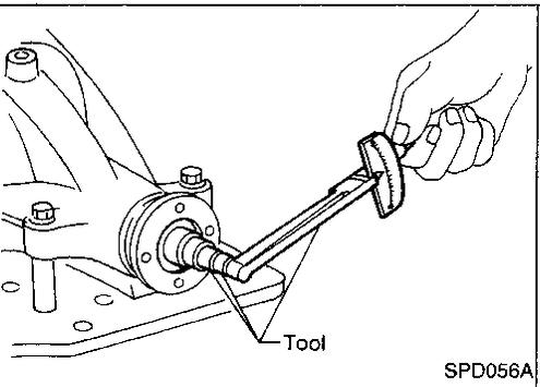
8. Turn drive pinion in both directions several times, and measure pinion bearing preload.
