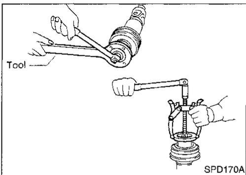
3. Remove locking nut with suitable tool.
