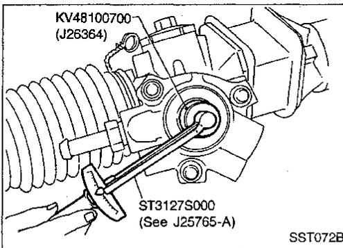
7. Measure pinion rotating torque within the range of 180° from neutral position.
