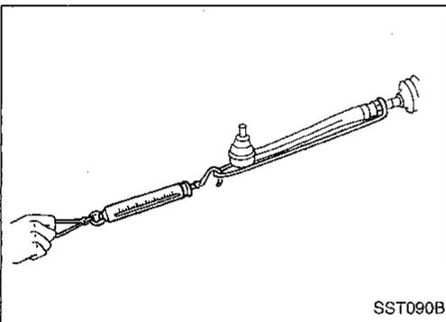
11. Check rack sliding force on vehicle as follows:
