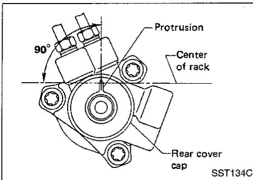
14. Ensure that the rack is centered. Install rear cover cap so that its protrusion is positioned as shown in figure.
