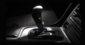
M-Atx' combines the driving ease of an automatic with the direct shifting of a manual. Shifting is either by the gear lever or by the toggle controls on the steering wheel.
