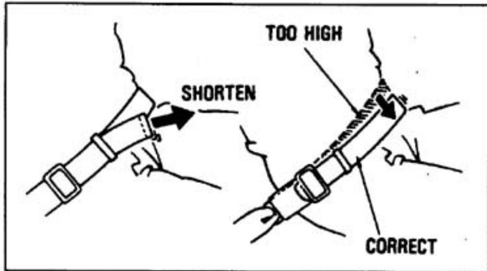
Remove excess length of belt and push the belt down over your hips.
