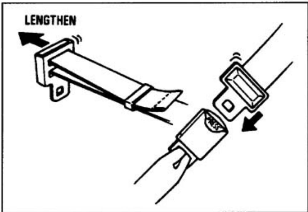
A line drawing showing a hand holding a seat belt tongue at a right angle to the buckle. An arrow points to the left, labeled "LENGTHEN". The buckle is shown with a "PRESS" button. The tongue is being pulled through the buckle.
