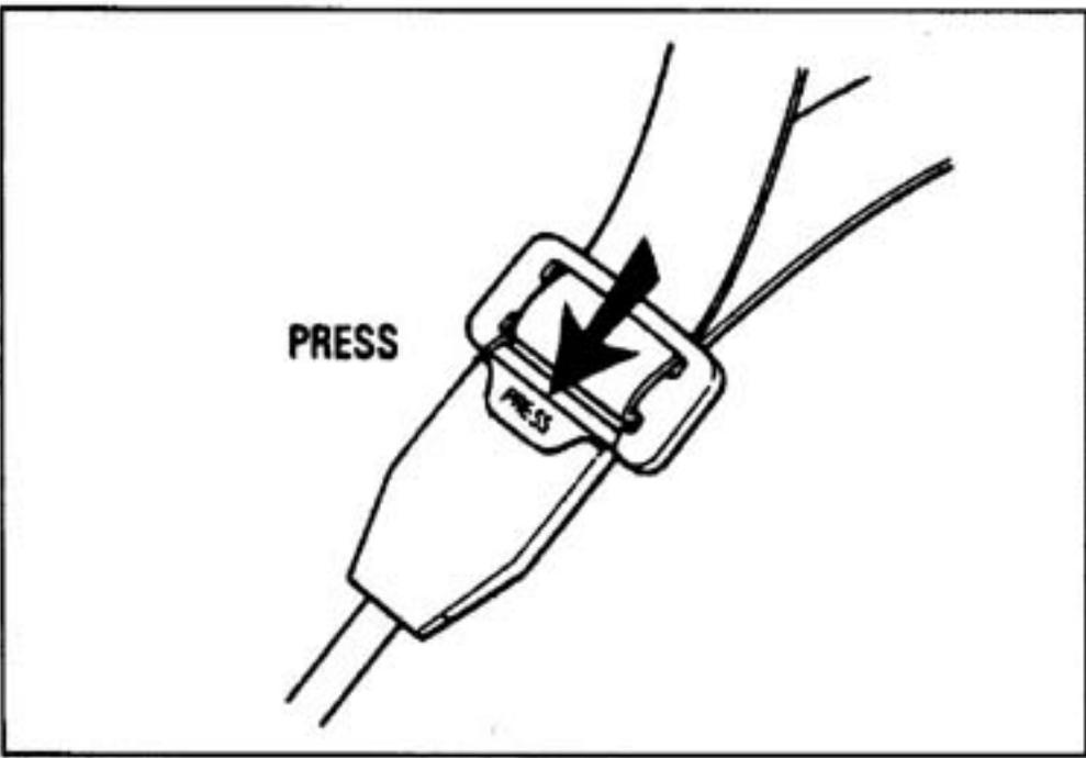
A line drawing of a seat belt buckle. A hand is shown pressing a button on the front face of the buckle. An arrow points to the button, and the word "PRESS" is written next to it. The buckle is attached to a seat belt strap.
