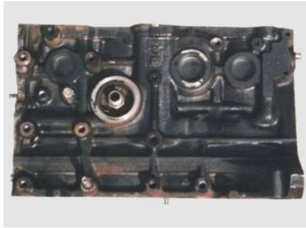
Exhaust side of 4A-G engine block. Top, 4A-GE, painted and cleaned ready for assembly; Middle, 4A-GEZ, U.S. model AW11; Bottom, 4A-GELU, Hi-comp. AE92. Notice the thicker horizontal stiffening rib just above the engine oil pan interface and the stiffening rib between the freeze plugs for added strength and stiffness.
