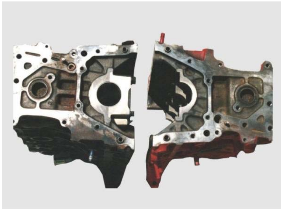
Front view comparison between a 4A-G normally aspirated block, right; with a later version AE92 Hi-comp 4A-GELU block, left. Notice the vertical stiffening rib extending from the water inlet opening to the main bearing saddles. Also notice the thicker main bearing saddles to give additional strength and stiffness.
